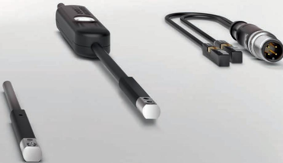
Our magnetic field sensors are used chiefly on cylinders and grippers for monitoring the piston position. The sensor thus recognizes the field of the magnet integrated into the piston through the actuator wall, even at high travel speeds.
