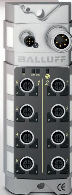
I/O blocks from Balluff connect binary and analog sensors and actuators to the control level via a bus. By using our modules you can significantly reduce the number of cables required. The Balluff I/O blocks also offer additional functions for signal preprocessing and expanded diagnostic options. Various form factors and connection technologies provide solutions for the widest range of requirements even under extreme ambient conditions.
