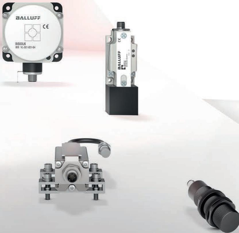
Our low-frequency RFID systems BIS L are suitable for applications that involve just the identification and require less data processing. For example, often only a (read-only) code is required for tracing. The 125-kHz systems function reliably up to ranges of 100 mm and are relatively neutral with respect to materials such as water, textiles, wood and aluminum.
