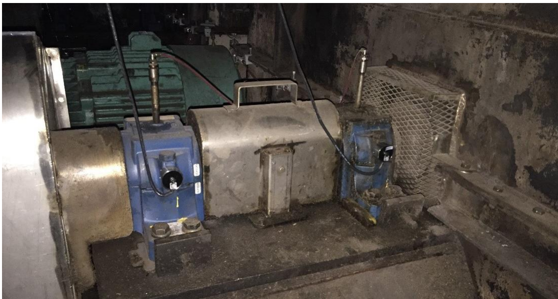
Figure 3: The Dynapar OnSite™ system shown with sensors mounted to both the inboard and outboard pillow-block bearing housings.
