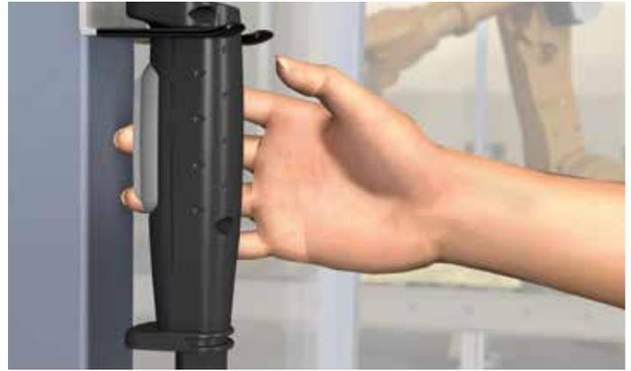
Manually operated safety control devices which, when continuously activated and used in conjunction with a separate actuating control, will allow the machine to function in manual operating mode. The handheld grip-styled switch is used for manual control of machine functions, including visual observations, minor adjustments, calibration and more.
