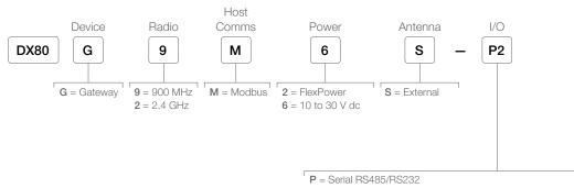
P2 = 4 Discrete IN, 4 Discrete OUT, 2 Analog IN, 2 Analog OUT
