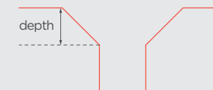
Determines the depth of the countersunk hole relative to the surface that the countersunk hole is on.
