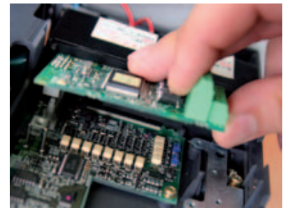
Connector system for time-saving installation
