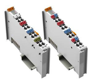
WAGO has developed variants of our filter modules that have built-in ground fault diagnostics. The 750-624/020-002 and 750-626/020-002 are able to monitor both the +24 VDC and 0 VDC supply connections for impedance to ground.
